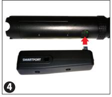
Connect the Smartport to the laser module section.
