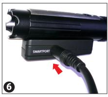
**Option 1>** Connect the AV cable to the Smartport.
