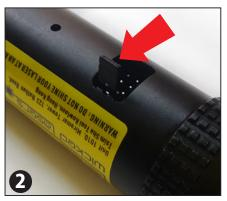
Remove the jumper shown here before connecting the Smartport.
